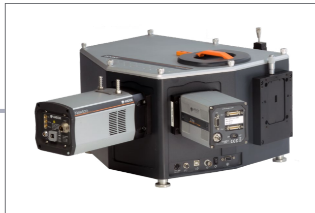
Kymera 328i with 300 l/mm grating, iVac 316 with high resolution 15 μm pixels, full vertical binning.
